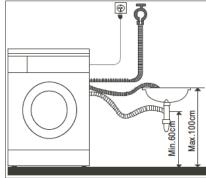
If you are positioning the outlet hose to drain into a sink or trough, please ensure that it is fixed in place and that the sink remains unblocked at all times.
