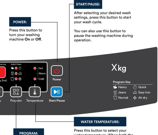
Press this button to select your wash program type. A solid indicator indicates the programs to the left, whereas a flashing indicator indicates the programs to the right.
