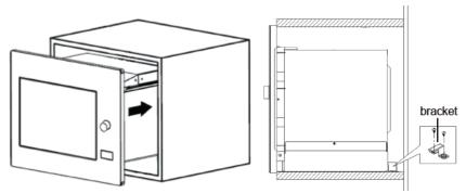
**4. FIX THE MICROWAVE IN TO PLACE** – Open the door and fix the microwave into place using Screw B, through the installation hole (indicated in the diagram below). Then fix the trim-kit to cover the installation hole.
