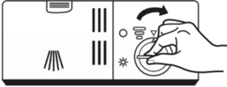
Figure 11- Re-fitting the cap onto the Rinse-aid dispenser.
