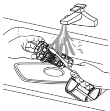
Figure 26- Rinsing and scrubbing any residual food particles or foreign objects from the filter components.
