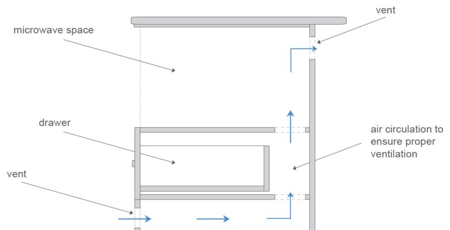
Note: Ventilation is critical for underbench installation also, either venting through the cabinet rear or down below the cabinetry (i.e. behind the kickboard).
